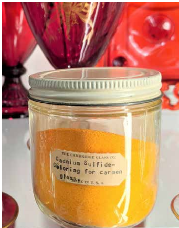
Cadmium Sulfide coloring for Carmen glass
